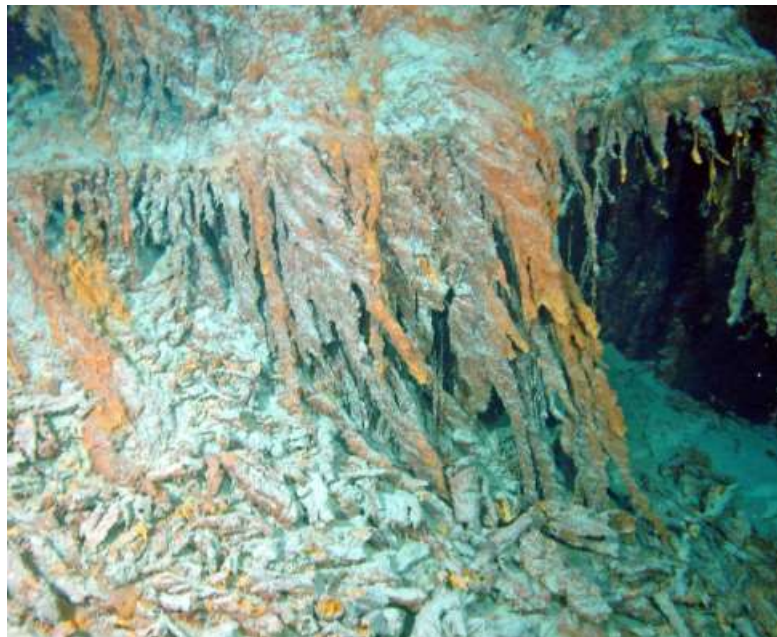
Rusticles showing the decay of the Titanic's hull: Wikipedia
